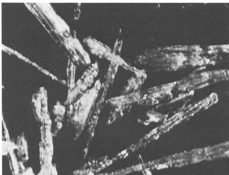
Fig. 1. Micrograph of acetamide (stable form), magnification, 7.5: 1.
